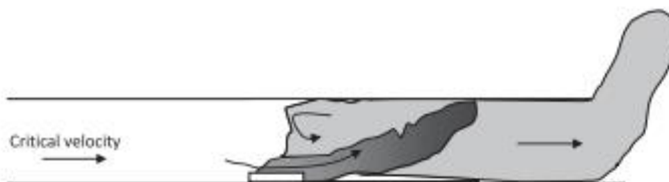
Fig. 12.4 A sketch showing a typical smoke stratification for group 3, i.e. a flow velocity larger than the critical flow velocity, u_c
